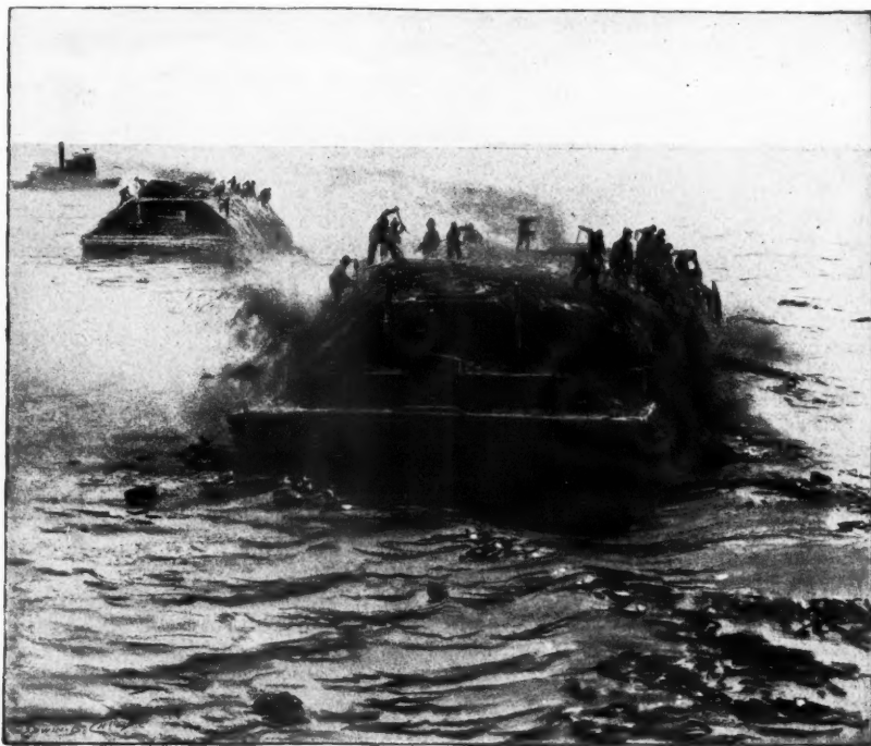
Former method of unloading ashes and rubbish from flat scow at sea. This material was often washed upon the bathing beaches.
